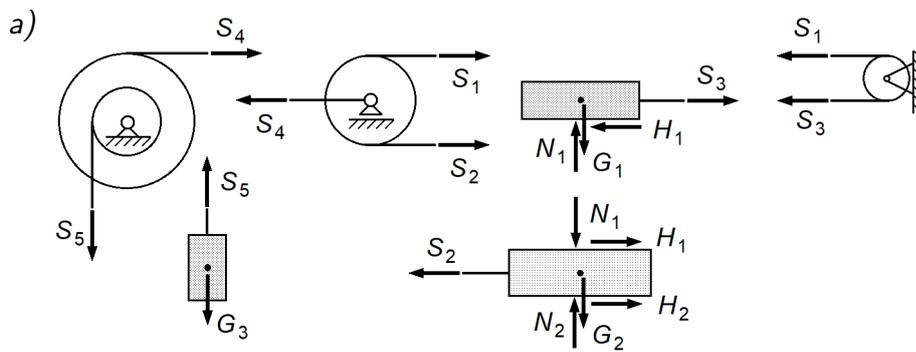
b)  $S_5 = G_3 = 400 \text{ N}$  ,  $S_4 = \frac{1}{2} S_5 = \frac{1}{2} G_3 = 200 \text{ N}$  ,  $S_1 = S_2 = \frac{1}{2} S_4 = \frac{1}{4} G_3 = 100 \text{ N}$  ,
